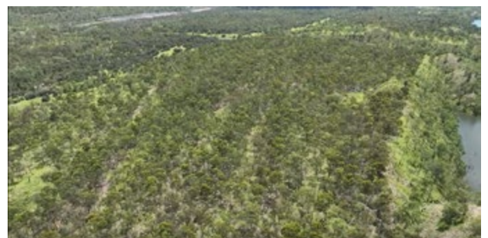
Figure 2 - A3 Mid Certified area - this area was rehabilitated in 1999 through recontouring and seeding spoil using the internally drained rehabilitated landform methodology. In this view it is delineated by A3 pit water storage (right of view) and Brigalow regrowth area (left of view). Intended post mine land use is open woodland. View captured via UAV 4/1/2024
